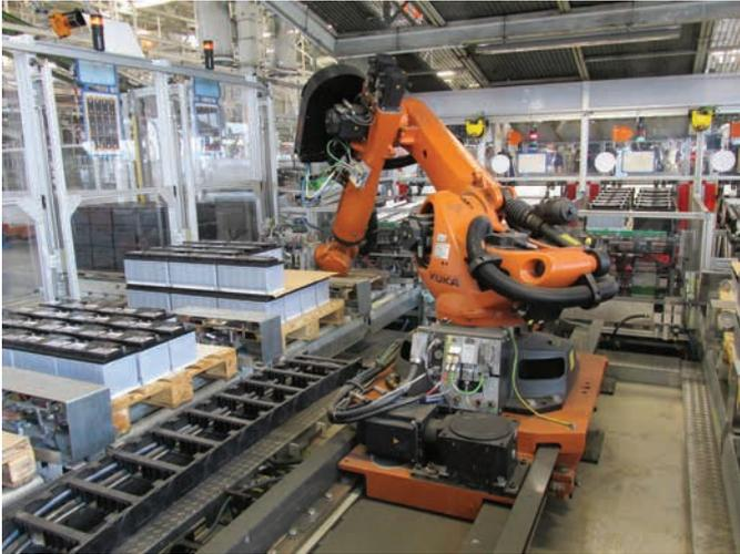
Battery assembly is used as the reference system, i.e. the first system that was built with PROFINET. The PROFINET-INspektor® is silently watching
